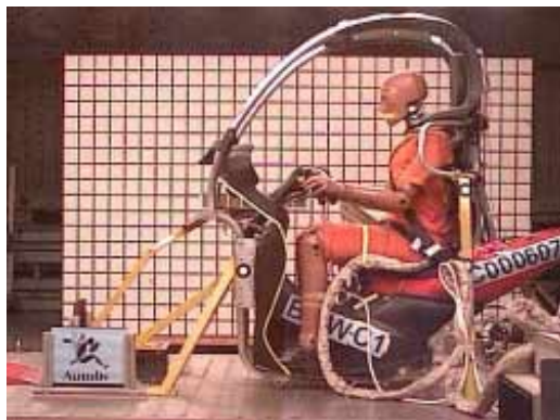
Figure 9. Sled test set-up
